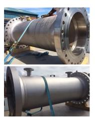
Protective coatings are applied on completion of the cleaning and inspection process in our controlled environment within in our facility, coatings can be applied by hand, conventional spray, pressure spray or we can use the latest technology from Graco in the Airless Spray System for the larger items or larger coats, such as fire protection. Multi coats systems are easily covered in house, all items are masked off in house to drawings and specification.
